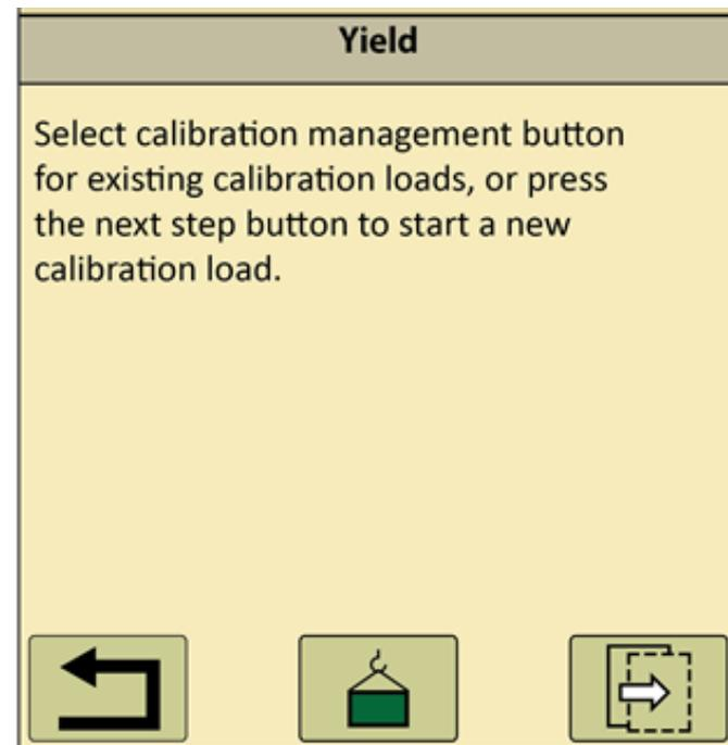
**4.** Select the “next” button to begin the calibration, be sure the grain tank is empty.
